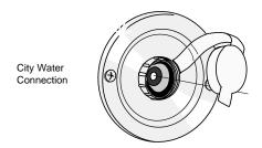
When connected to an outside source of water, the water bypasses the demand pump and storage tank and supplies pressure directly to individual faucets and toilet. A check valve built into the pump prevents water from entering the pump and filling the storage tank.
