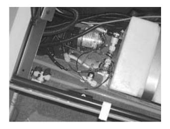
**Model 22FD:** The drain valves are located below an access hole beneath the bedboard of the rear bed in the left (driver side) rear of the coach. Lift or remove the bed mattress to expose the access hole.
