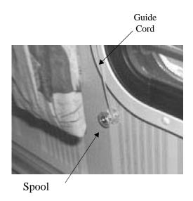
To loosen the tension, unwrap the guide cords from the spools one turn at a time until desired tension is achieved.
