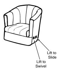
**Swivel:** Pull up on the swivel lever located on the lower left hand side of the seat. The seat will lock into place whenever it reaches the center aisle facing position.
