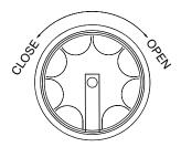
If the window will not open after three or more full turns of the knob, the glass may be stuck to the sealing gasket. Go to the outside of the coach and gently free the glass with your fingers. A periodic light dusting of talcum powder on the gasket should prevent this from recurring.
