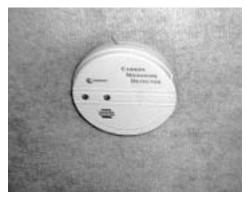
The CO alarm is powered by a 9-volt battery and contains a sensor that is designed to detect toxic carbon monoxide gas fumes resulting from incomplete combustion of fuel. It will detect CO gas from any combustion source such as the furnace, gas range/oven, water heater, refrigerator, chassis engine, and electric generator engine.
